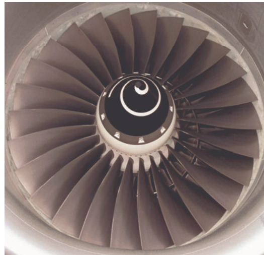
Figure 4. A Trent 800 fan set comprising 25 blades. The fan has a diameter of approximately 3 m and the mass flow of air through the engine is approximately 72 tonnes/min, or 1.2 tonnes/second.
